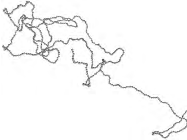
Figure 5.19. Illustration of a polymer as a random walk. To prepare this figure, each segment was permitted to turn at an angle up to 26^\circ relative to the previous segment.
