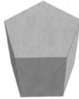
Figure 2.15. A solid may have pentagonal symmetry, but one cannot tile the plane with it, so one cannot build a lattice with this symmetry.
