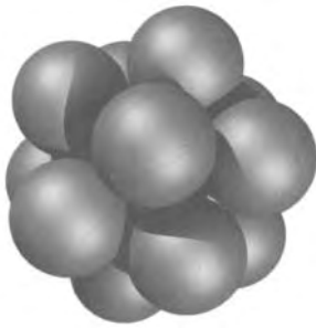
Figure 5.30. Twelve neighbors symmetrically arranged about a sphere form an icosahedron.
